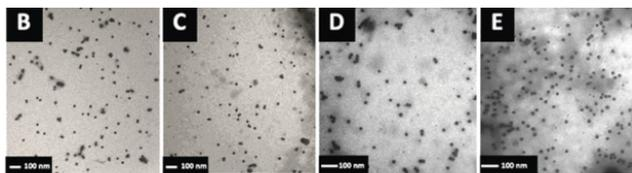
TEM images of  $Fe_3O_4@OA$  (B),  $Fe_3O_4@CTA$  (C),  $Fe_3O_4@PEG$  (D) and  $Fe_3O_4@PEG@AD$  (E) magnetic nanoparticles.
